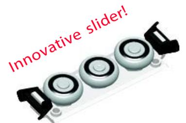
The contoured rail comes in lengths up to 3 meters (9'10"). The raceways are internal for better protection and compactness. The rails come with standard mounting holes with a hole pitch of 80mm (3.15"). The steel rollers have 2Z sealing and are lubricated for life. These rollers have eccentric pivots that allow adjusting the preload when mounted inside the rail.
