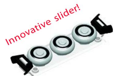
The contoured rail is made of AISI316L stainless steel and comes in lengths up to 3 meters (9'10"). The raceways are internal for better protection and compactness. The rails come with standard mounting holes with a hole pitch of 80 mm (3.15"). The rollers have double seals (2RS) and are lubricated for life. These rollers have eccentric pivots that allow adjusting the preload when mounted inside the rail. The rollers are mounted to the slider body in AISI316L stainless steel.
